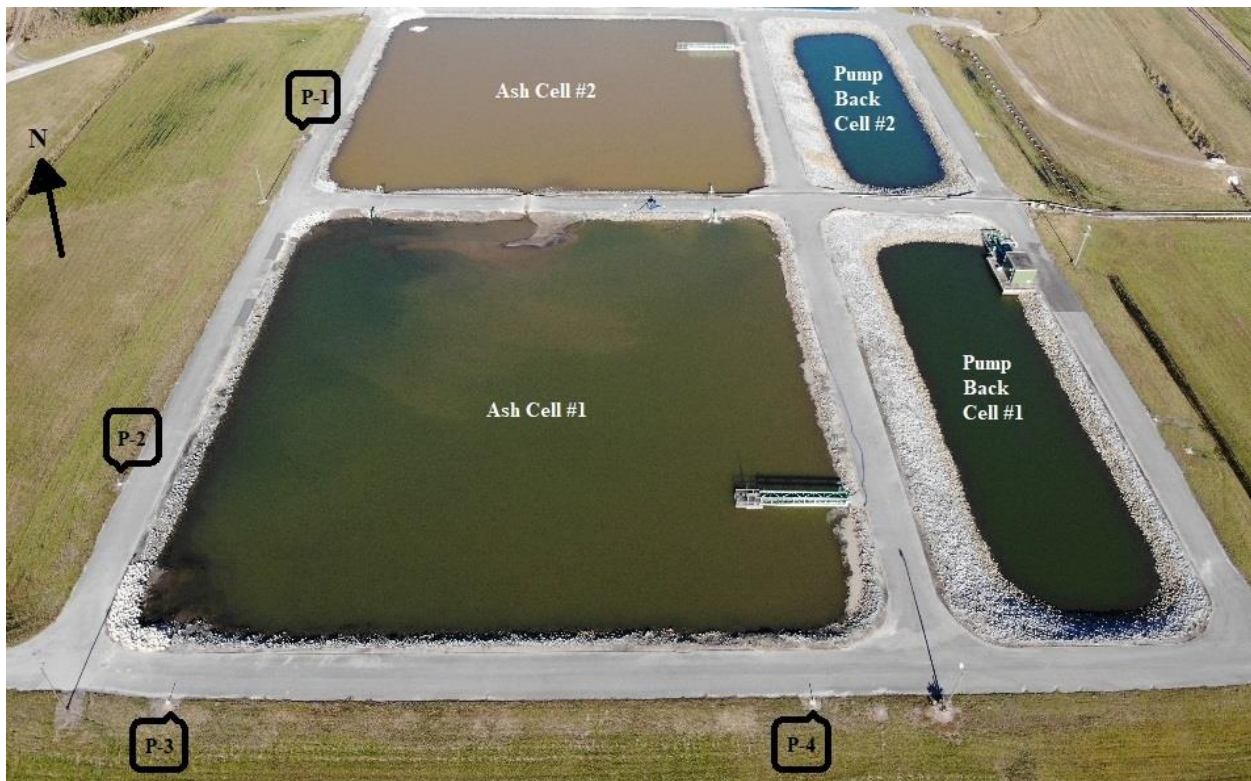
Figure 1. Layout of the CCR Surface Impoundment System and Adjacent Pump Back Ponds (IWCS 2018a)
